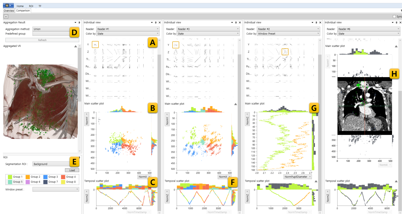
Fig. 5. GazeDx interface for chest normal case ( Comparison tab). (A) Scatter plot matrix. (B) CIS: context-embedded interactive scatter plot with gaze points grouped to five clusters. (C) Interactive temporal chart. (D) Aggregation pane showing aggregated gaze data for the readers in individual view panes. (E) ROI selection pane with “Segmentation ROI” filter and “Window preset” filter. Interactive temporal charts in (C) and (F) clearly show the difference in gaze pattern between scanner and driller strategy (frequently changing color in (C), scanner; relatively consistent color in (F), driller). (G) CIS with horizontal axis of pupil diameter and vertical axis of slice index, where the gaze data is color-coded by window preset (left-shifted green cluster for lung, and right-shifted orange cluster for mediastinum setting). (H) CIS with embedded coronal plane image.
