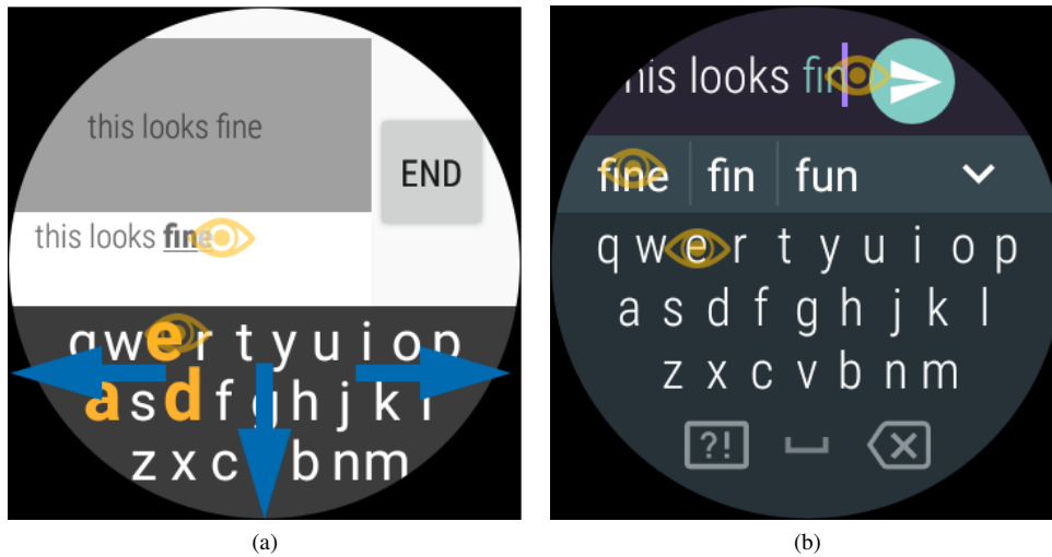
FIGURE 2: The virtual keyboard layout is shown in the circular smartwatch; (a) our soft keyboard (VHA) and (b) Google Keyboard (Gboard) on Android Wear 2.0. Possible gaze points to enter a word are depicted with a yellow eye icon. The VHA keyboard on the left shows additional information, such as a presented phrase for the user experiments in the gray textbox located at the top. On the right side, there is the end button, which is used to finish entering a phrase. The input textbox is located below the gray textbox showing the input words as well as a predicted word. The cursor is located as a blinking underline at the end of the actual input text. At the bottom of the soft keyboard, there is a QWERTY layout to enter characters. Bolded yellow keys are predicted character candidates for the next input. The blue arrow means swiping gestures. The left arrow means swipe-left gesture acting as a back key, and the right arrow means swipe-right gesture acting as a spacebar, and the down arrow means swipe-down gesture triggering a word completion. The Gboard on the right has no area to show information at the top. Instead, the input textbox is located at the top showing last input words, and at the end of the input textbox, there is a blinking cursor as a vertical bar. On the right side of the input textbox, there is a rounded button to finish entering a sentence. Below the input textbox, the suggestion bar shows suggested words for fixing or predictive typing. Users can see more suggested words by touching the downward arrow button. Below the input textbox, the QWERTY layout is shown to enter characters on top of the special keys for mode change, spacebar, and back key.
