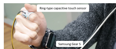
Figure 1. Samsung Gear S detects wrist rotation and ring-type capacitive sensor detects touch gestures.
