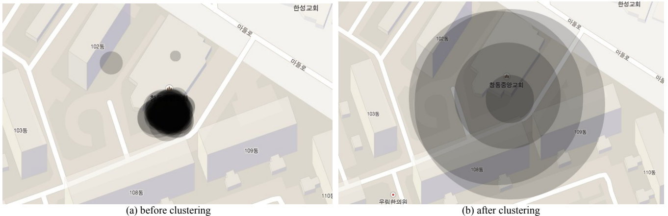
Fig. 3. Clustering GPS data. Before clustering the GPS data, it is difficult to identify each circle since many circles overlap in a small area. After clustering the GPS data, the scattered circles are clustered and made into a few big circles.
