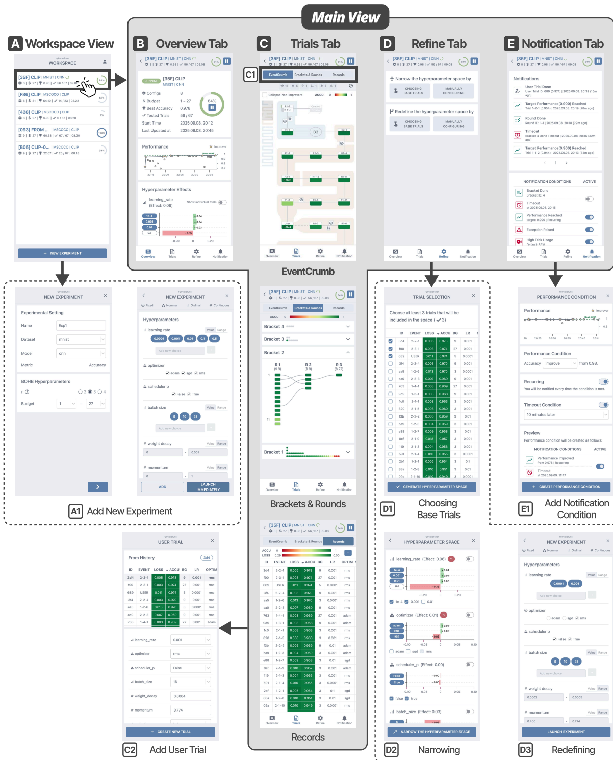
Figure 5: The HyPockeTuner interface, consisting of the Workspace view (A), where users select an experiment to inspect from the list, the Overview tab (B), the Trials tab (C), the Refine tab (D), and the Notification tab (E). In the Trials tab, users can switch between three viewing modes: the EventCrumb mode, the Brackets & Rounds mode, which presents trials in the bracket-round hierarchy, and the Records mode, which provides a traditional tabular representation.
