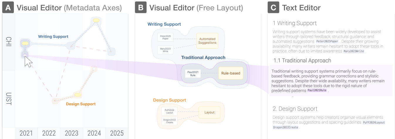
Figure 1: Conceptual overview of CrossLIT, a literature review supporting system where visual and text editors are connected. In the visual editor, users can examine (A) metadata such as venue, year, and citation relationships or (B) arrange papers in a free layout according to their interpretation. In the text editor, users can (C) compose the manuscript directly.
