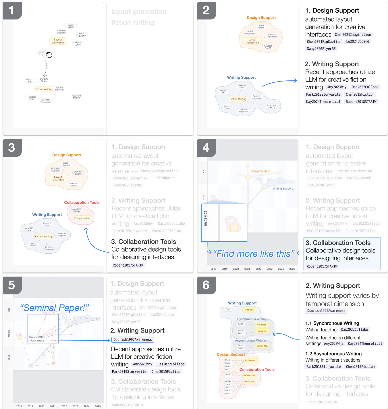
Figure 2: An example scenario of using CrossLit. (1) The user sorts papers into piles and adds short notes in the visual editor. (2) The user makes groups from the piles in the visual editor, and the system drafts a section for each group in the text editor. (3) The user writes a new section in the text editor, and the system creates a corresponding group in the visual editor. (4) The user organizes papers by venue and year in the visual editor. The user identifies the need for new papers from both editors. (5) Among the newly discovered papers, the user discovers a seminal work through citation patterns in the visual editor. (6) The user restructures sections into subsections in the text editor, and the visual editor updates accordingly.
